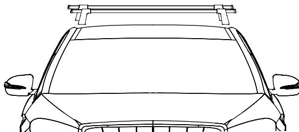
$$\text{[Icon of a roof rack]} + \text{[Icon of a bag labeled 'xx Kg']} = \text{Max 50 kg}$$
